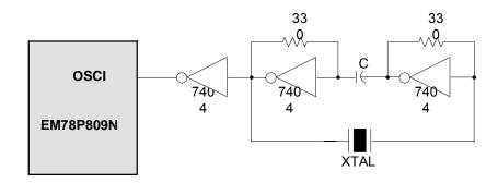
Fig. 32. Crystal/Resonator-Series Mode Circuit
